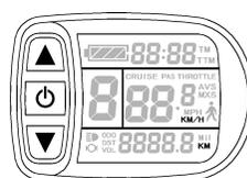
The metric units will be set after finishing setting wheel diameter, Km/H and Km flash. Hold ▲ or ▼ shortly and select the three metric units of speed, mileage, and ambient temperature in synchronization.
