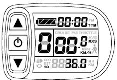
Hold ⏻ button shortly in display 2 to enter display 3. In the riding condition, five seconds later, a single maximum speed (MXS) display automatically returns to the real riding speed (Km/H).
