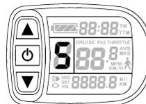
Hold or shortly to switch 1-5 file gear. Gear 1 is for the minimum power, gear 5 is for the highest power. Each startup will automatically restore the gear shutdown last time(the user can set randomly). Gear 0 is without booster function.
