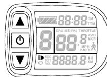
Hold long to turn on backlight and headlights (the controller should have headlight drive output function); hold long again to turn off the backlight and headlights.
