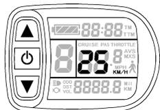
After power on for 5 seconds, hold ▲ and ▼ at the same time, and maximum riding speed Km/H and MXS flash, ▲ or ▼ shortly to set the maximum riding speed (default 25Km/H). ⏻ button shortly and Hold go to the next parameter settings.
