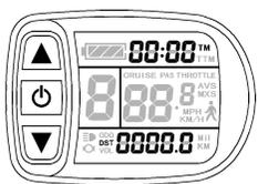
After power on for 5 seconds, hold ▲ and ▼ at the same time, single trip riding time (TM) and single trip distance (DST) flash, hold ⏻ button shortly, the content of both is cleared. If failed holding the button within 5 seconds, it will automatically return the display interface after 5 seconds, original content is preserved.
