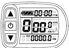
Hold ⏻ button shortly in display 1 to enter display 2. In the riding mode after 5 seconds, display 2 automatically returns to display 1.
