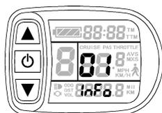
Electronic control system failure will display (flashing) fault code. Once the fault was removed, it automatically exits from the fault code display interface.
