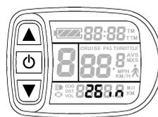
The wheel diameter will be set after finishing setting the maximum riding speed, wheel diameter specifications flashes. Hold ▲ or ▼ shortly to set the specifications of wheel diameter. Select the range 6,8,10,12,14,16,18,20,22, 24,26,700c and 28 inches. Hold ⏻ button shortly and go to the next parameter settings. **FIREFLY WHEEL IS SET FOR 12" WHEEL DIAMETER.**
