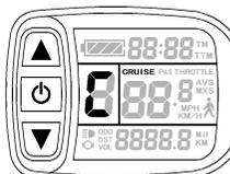
After the cruise function is turned on, the trip riding speed is greater than 7 km/ h, hold long and enter cruise, the CRUISE lit. Brake or hold any button to cancel.
