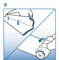
Fold and roll up the device as shown starting at the point furthest away from the valve. Continue until all the air is expelled. Clean the device and allow to dry.
