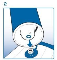
Connect the valve on the pump to the valve on the device -Push fit.
