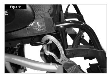
Position of the Front tie down restraint., (Fig.4.11).
