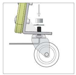
**02a** Use allen key to insert bolt up through the caster and bracket. Tighten nylon nuts with a crescent wrench. Note: Maintain tight screws.
