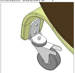
**02** Be sure casters w/break are installed toward rear of base. This increases base strength.
