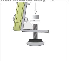
**03** Feed Non mobile glide up through base bracket. Install lock washers then nut. Note: Maintain tight screws.
