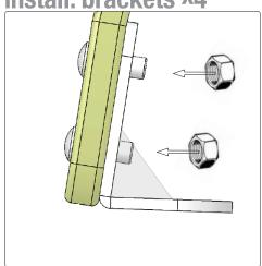
**01** Bolt metal bracket to Wooden Base x4. Note: Maintain tight screws.
