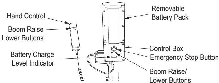
When the power pack needs charging, it can be removed from the lift and fitted to an off board charging unit. The battery charge level is displayed by the indicator on the control box.
