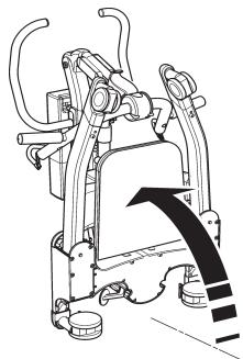
**NOTE:** If you wish to separate the mast and boom completely from the base and legs, undo the mast-locking lever fully (remove pin assembly from mast) and lift the mast and boom completely free from the base. Be careful not to lose the mast lock lever and location spindle.
