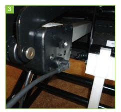
Disconnect the handset plug from the control box.
