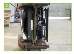
With two people, lift the chair onto a trolley on its side (not the side with the handset).
