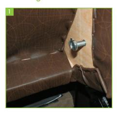
From the inside of the backrest, remove the screws securing the backrest brackets.
