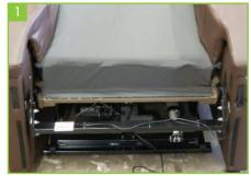
Remove backrest – remember to remove the screws securing the backrest brackets on the inside of the backrest.
