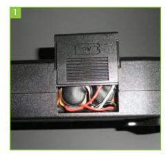
The transformer is fitted with a battery backup which allows the chair to be lowered in the event of a power failure. Replace the batteries by removing the small plastic cover on the side of the transformer.
