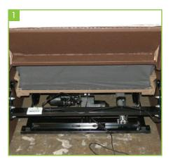
Line backrest up as close as possible to the backrest brackets (it may sometimes be necessary to bend the brackets on the mechanism inwards slightly).
