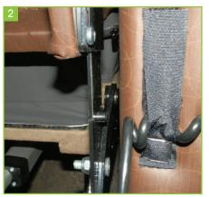
Insert one side of the backrest at a time, taking care to make sure the backrest remains square and upright.
